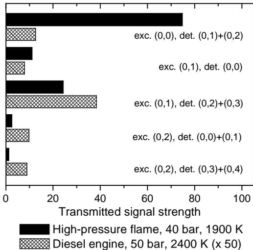
Fig. 3: Calculated signal strengths after laser and signal absorption by hot  $\text{CO}_2$  and  $\text{H}_2\text{O}$ , normalized to the (0,0) strategy signal without absorption. Exc.: excited, det.: detected vibrational band within the NO A-X system.
