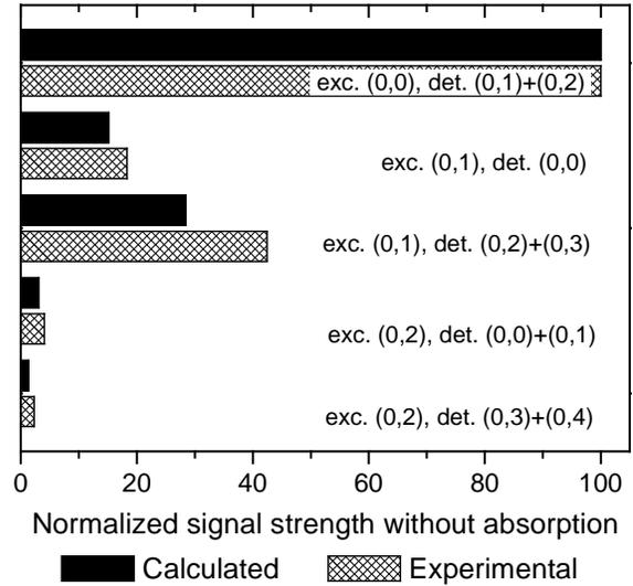
Fig. 2: Calculated and experimental signal strengths for the 10 bar flame. Exc.: excited, det.: detected vibrational band within the NO A-X system.
