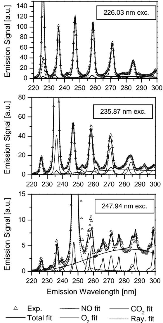
Fig. 1: Examples of the nonlinear least-square fit of simulated NO,  $O_2$ ,  $CO_2$ , and Rayleigh emission spectra (represented as Voigt line shapes) for the investigated excitation strategies at  $p = 60 \text{ bar}$ ,  $\phi = 0.83$ . The intensity is on the same scale in all panels.
